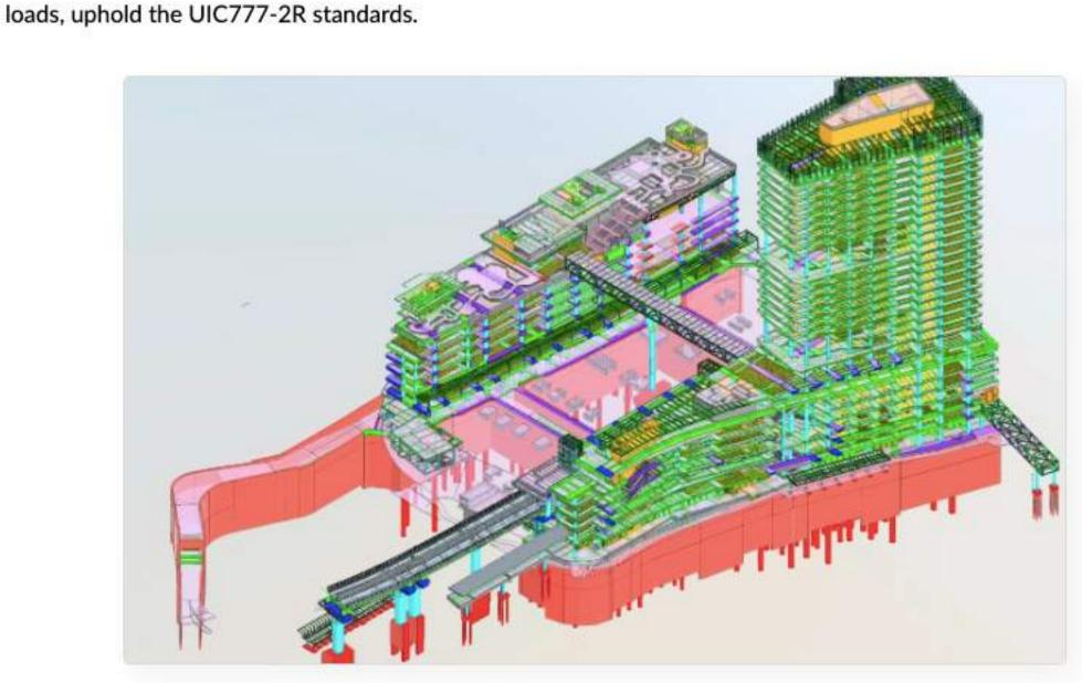
An extensive track-structure interaction analysis was conducted adhering to UIC774-3R guidelines, taking the use of FST into account. The design of the viaduct is intricately intertwined with its construction sequence, the roof structure above, and the building structure below. The viaduct's substructure is seamlessly connected to the building structure, with the pile cap forming an integral part of the B2 basement slab and the diaphragm wall of the West Wing structure.
